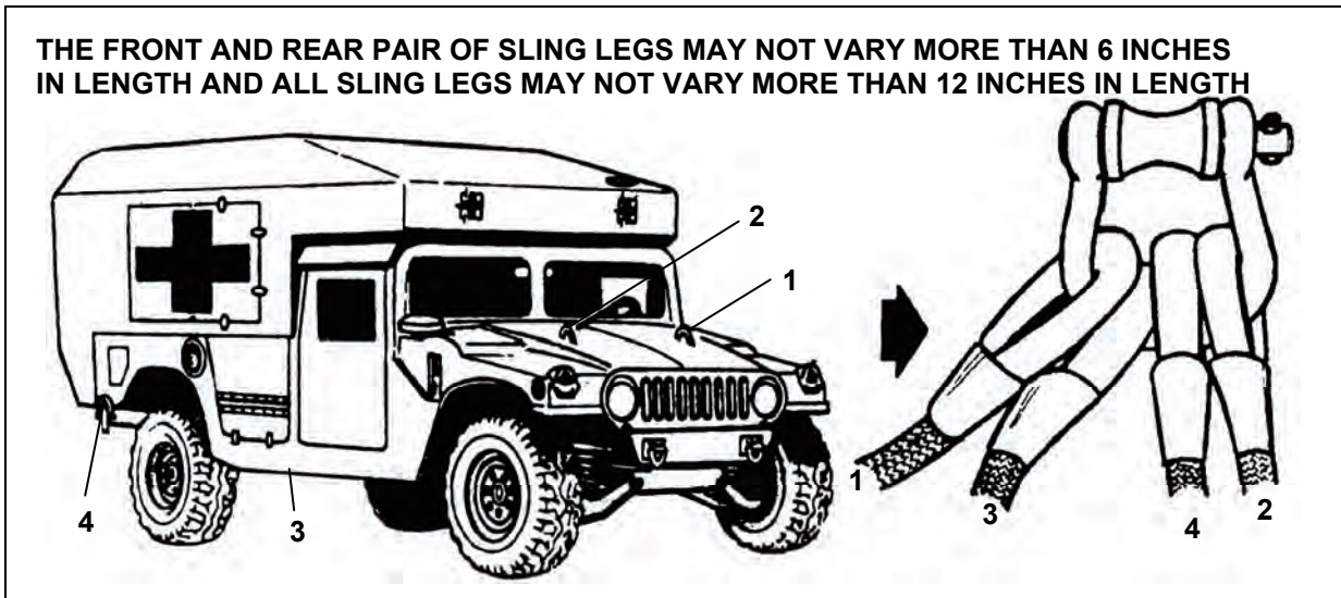
Figure 6-12. Load with Four Lift Points
